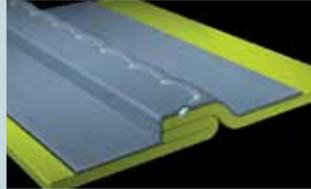
A heat sealed seam is sewn and then sealed with a heat activated tape. This method provides liquid proof seams, and is especially useful for Level A and B chemical protective clothing.
