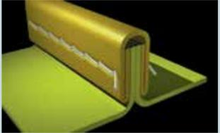
A bound seam joins two pieces of material with an overlay of similar material and is chain stitched through all layers for a clean finished edge. This provides increased holdout of liquids and dry particulates.
