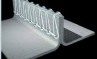
A serged seam joins two pieces of material with a thread that interlocks. This is an economical stitching method for general applications. This stitching method is generally not used for chemical protective clothing. It is more commonly found on disposable clothing where dry particulates are a concern.
