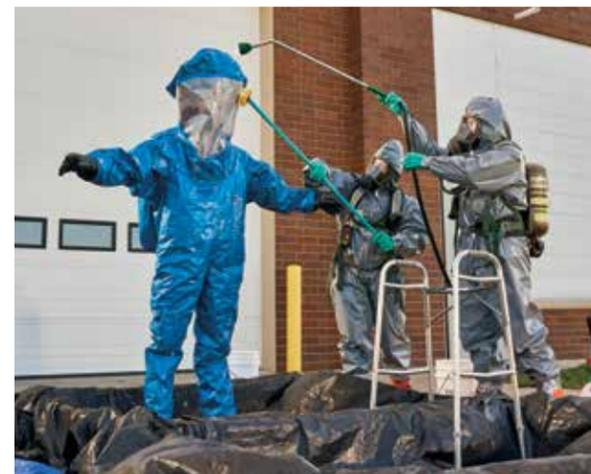
PTFE visor process permanently seals the visor into the suit with no sewing involved so that liquids can't penetrate the visor edge
